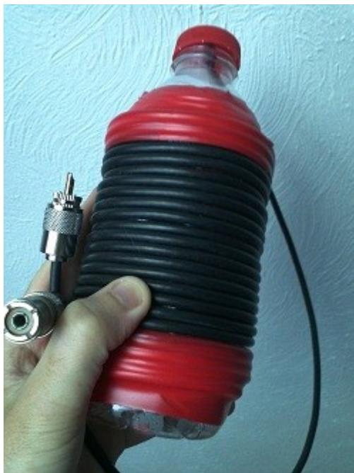
There are many other sites online that detail how these are made - any non-conductive material can be used as a former: water bottle, waste pipe etc. You can even mount 2 screw-hooks through the plastic and use it as a dipole centre!
